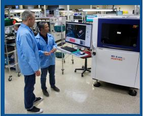
Matt McMillan from Silvercar by Audi and Richard Tsukano from East/West Manufacturing Enterprises review board quality using an Automated Optical Inspection (AOI) machine.
